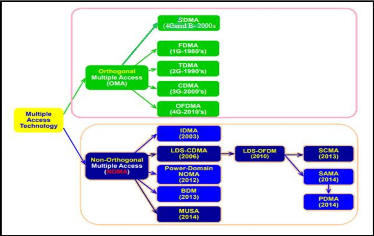
Figure 2.3: The Milestones Developments of Multiple Access (Dai et al., 2018)
