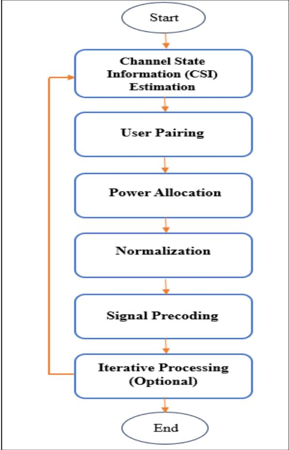
Figure 3.5: The Block Diagram for Proposed PA- NOMA Algorithm for Basic Steps
