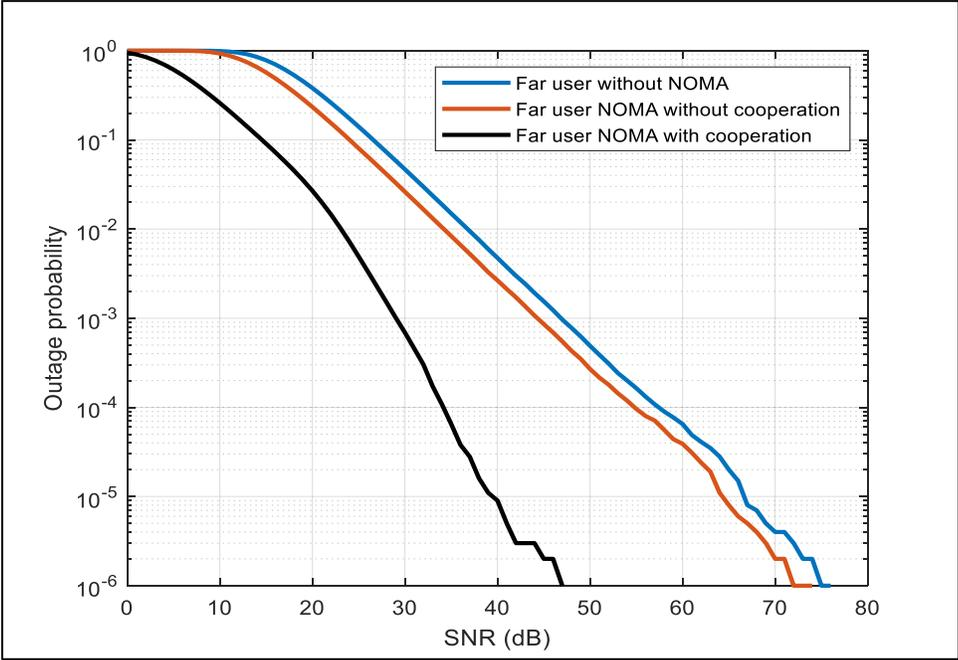
Figure 4.5: A Comparison of (OMA), (C-NOMA), and (Non-C-NOMA) for the outage probability versus SNR (dB)
