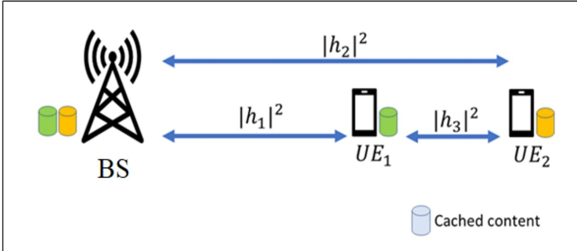
Figure 3.8: The System Model for C-NOMA with Caching
