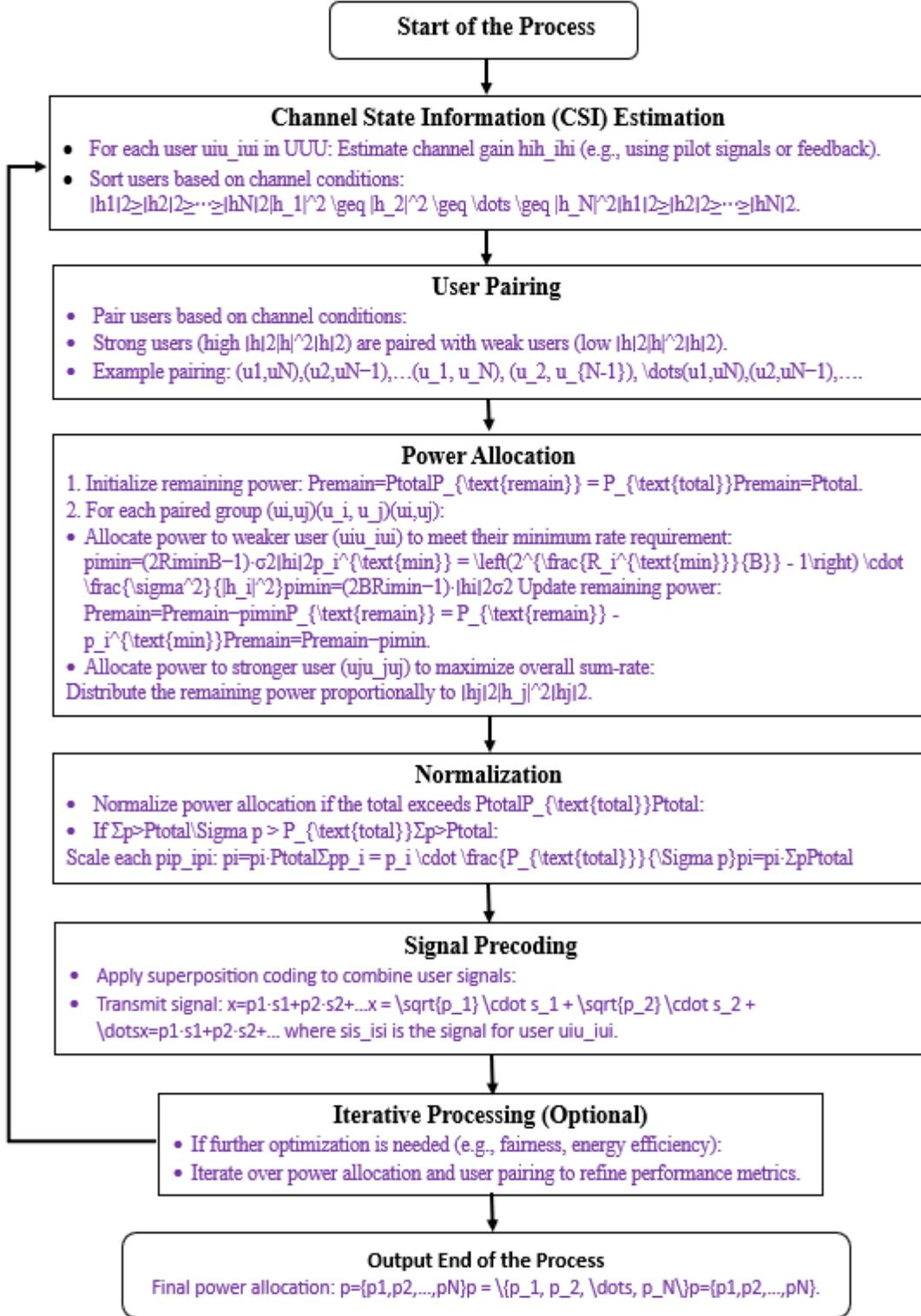
Figure 3.6: The Flow Chart for Process of Proposed PA- NOMA Algorithm for Basic Steps
