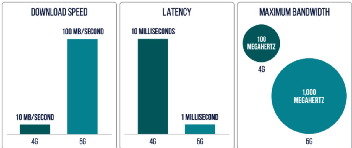
Figure 2.1: The Need for 5G Technology (Lal et al., 2021)
