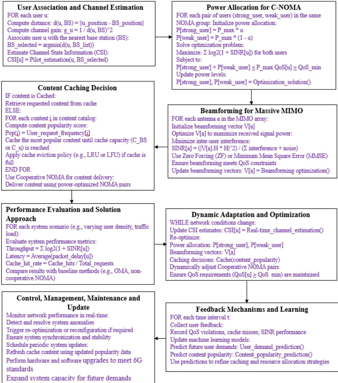
Figure 3.12: The Flow Chart for C-NOMA m-MIMO with Caching Proposed Algorithm in the 6G Mobile Communication Network System
