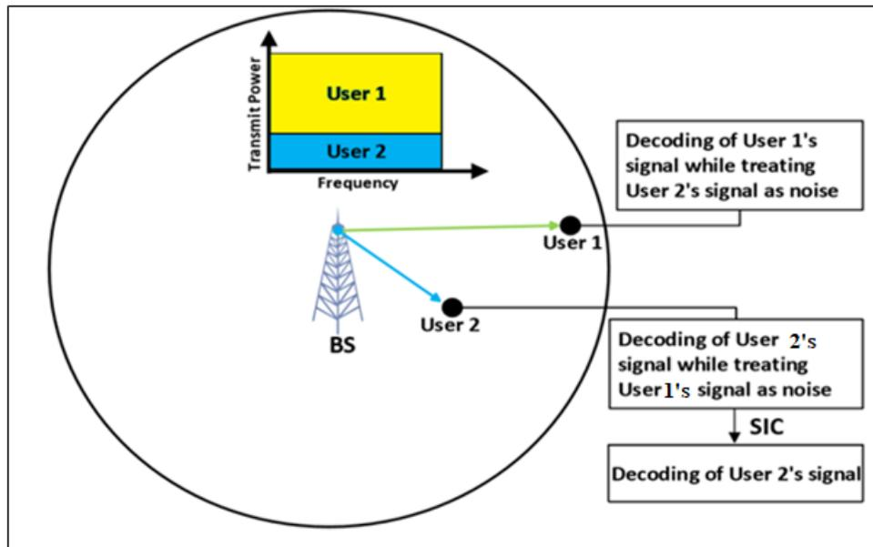
Figure 3.4: DL PA-NOMA System for two-users
