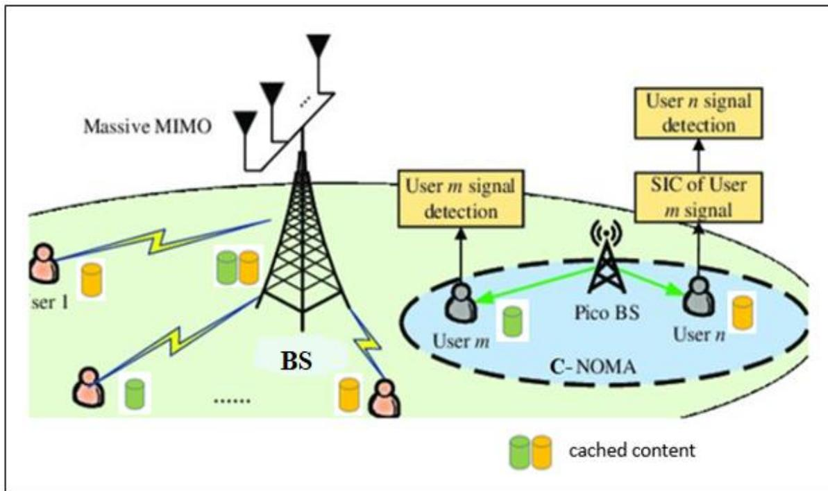
Figure 3.11: The System Model for C-NOMA Massive MIMO with Caching
