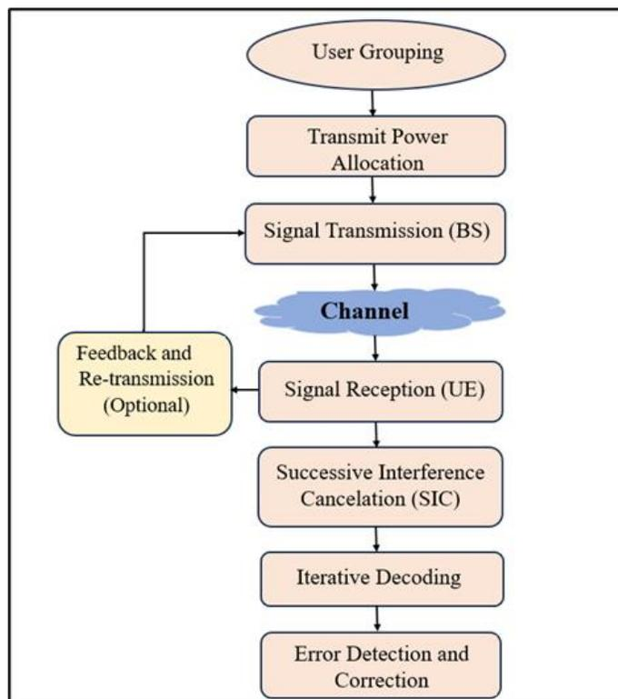
Figure 3.2: The Block Diagram for Proposed Process of a High-level Overview of the C-NOMA SIC Algorithm
