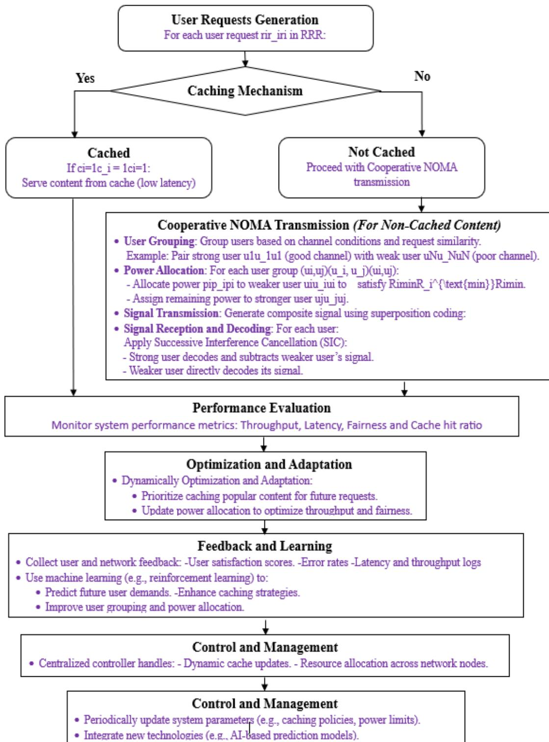
Figure 3.9: Flow Chart for C-NOMA with Caching Proposed Algorithm in the 6G Mobile Communication Network System
