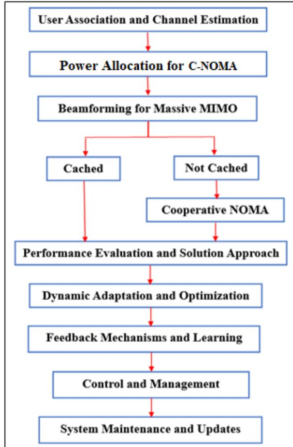
Figure 3.10: The Block Diagram of C-NOMA m-MIMO with Caching Proposed Algorithm in 6G Mobile Communication Networks
