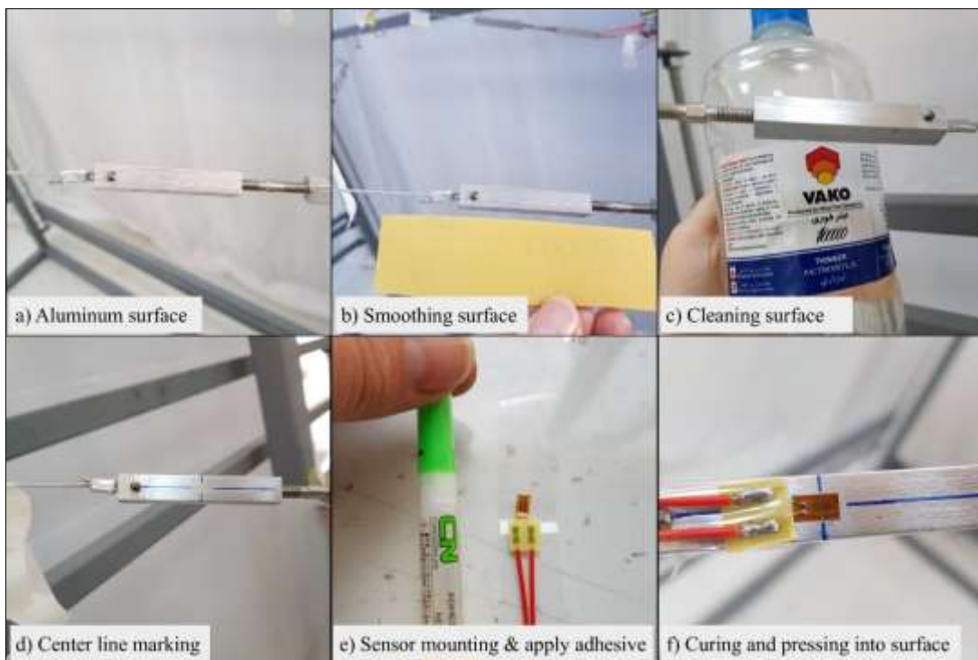
Fig. 4-17 Photo illustrating steps for strain gauge sensor placement
