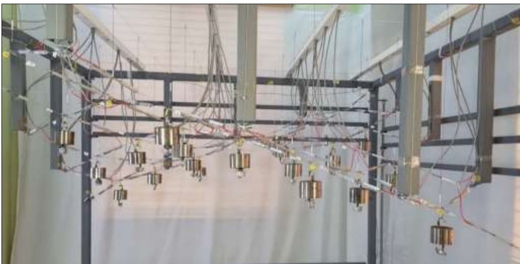
Fig. 5-5 Experimental model under vertical joint loads
