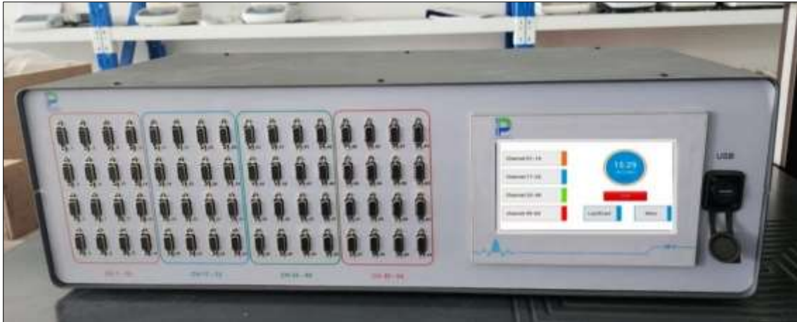
Fig. 4-16 64-channel data logger for strain measurement
