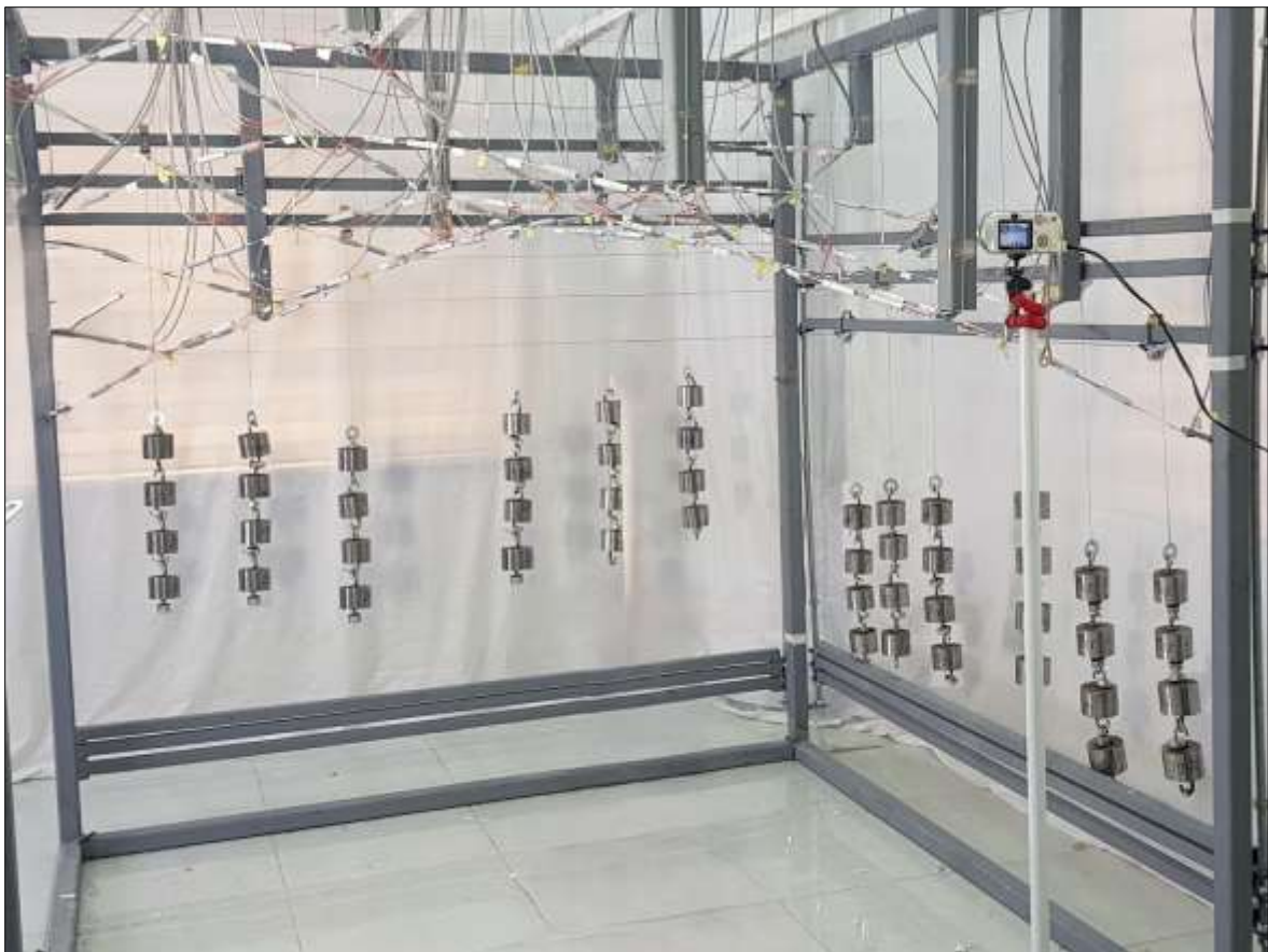
Fig. 5-7 Experimental model under horizontal joint loads
