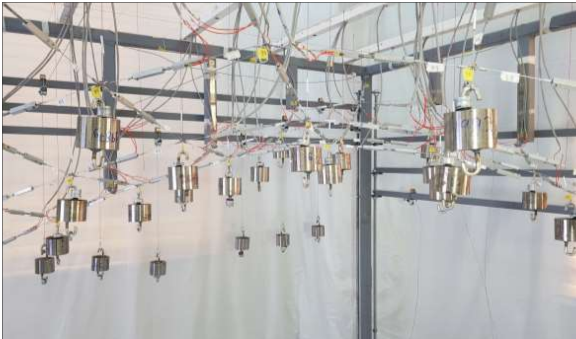
Fig. 5-9 Experimental model under vertical and horizontal joint loads
