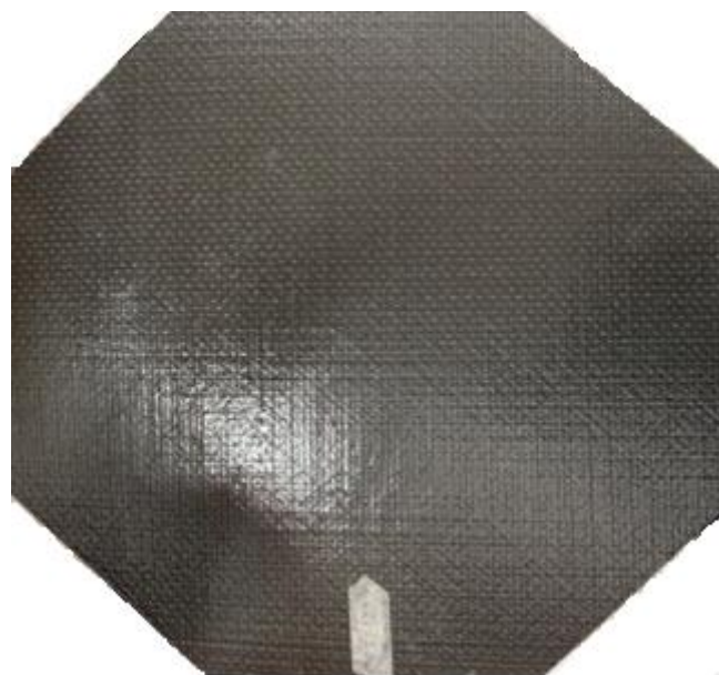
Figure 4-14 Unidirectional glass/carbon quasi-isotropic laminate
