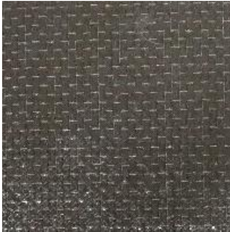
Figure 4-17 Unidirectional Glass/carbon cross-ply laminate
