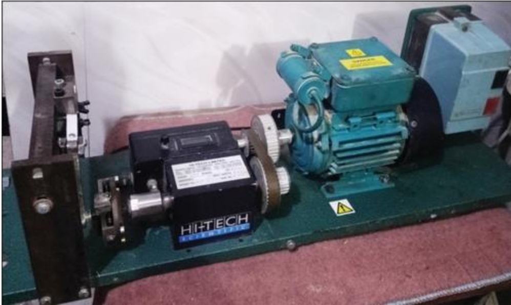
Figure 4-22 HSM20 alternating bending fatigue machine
