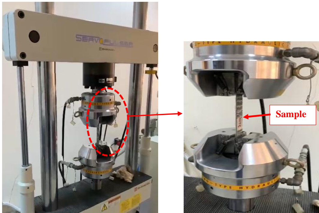
Figure 4-20 Shimadzu brand Servo-Hydraulic Fatigue Tester
