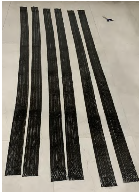
Figure 3.5: 10 cm width CFRP sheets to strengthen column ends
