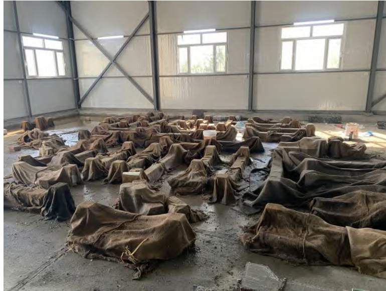
Figure 3.13: Curing process for columns and control specimens in room temperature
