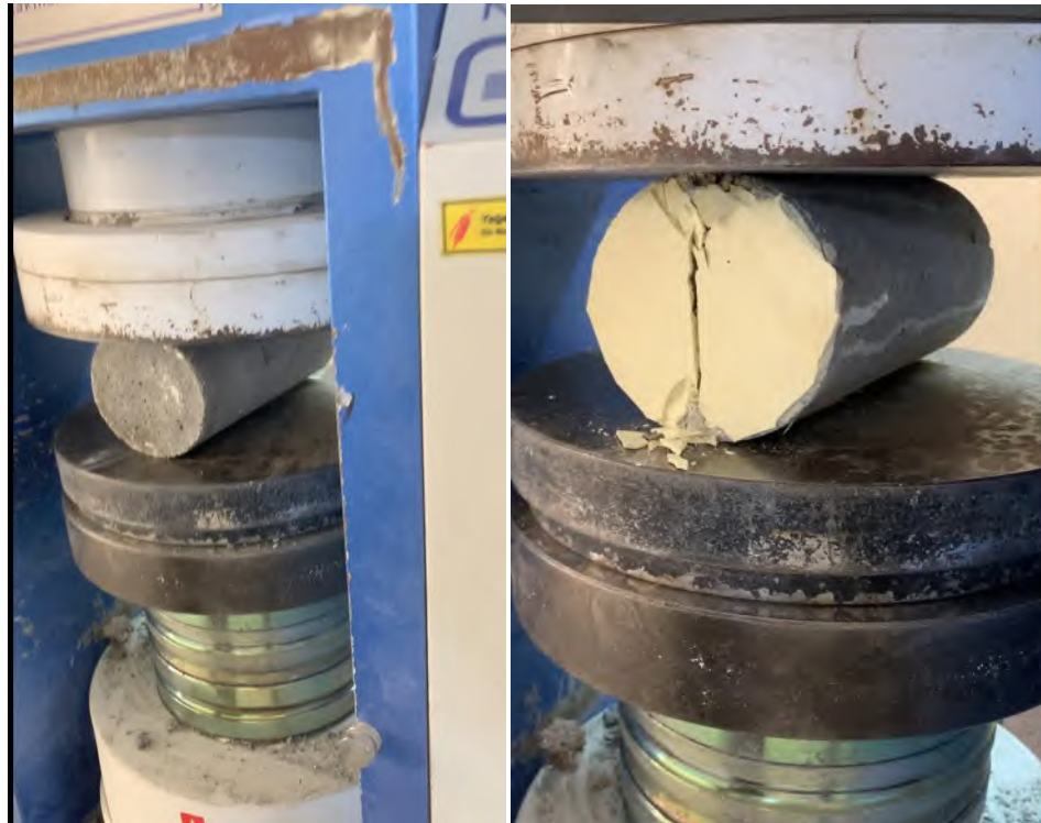
Figure 3.24: Hydraulic compression machine used for splitting tensile strength
