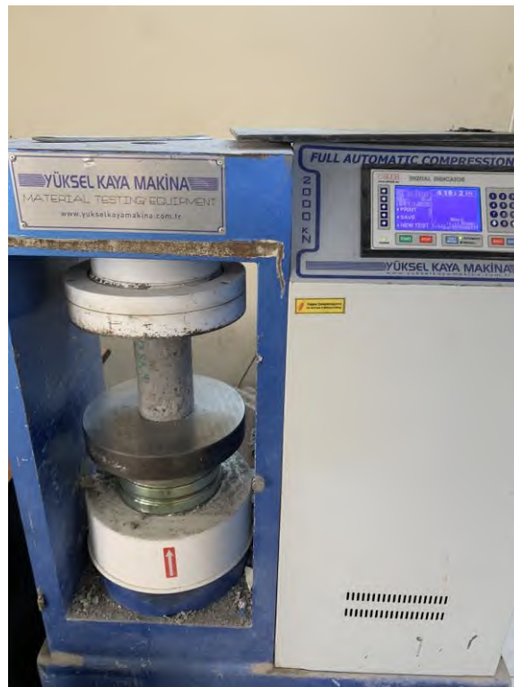
Figure 3.23: Hydraulic compression machine used for the compressive strength
