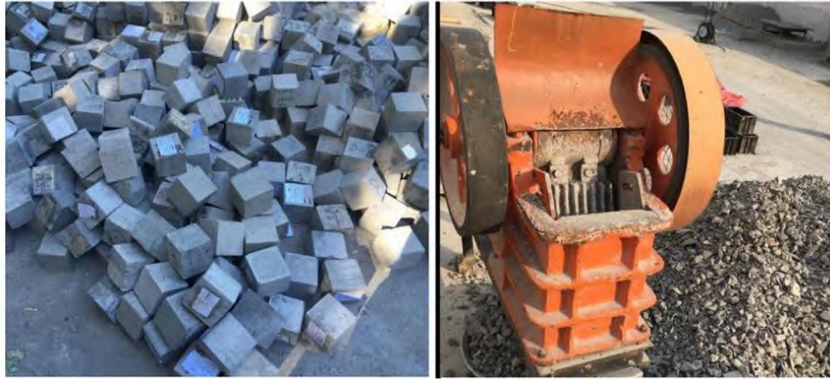
Figure 2.1 Waste concrete blocks (Right) and jaw crusher (left) Gao et al. (2021)
