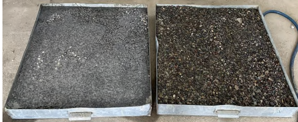
Figure 3.9: Coarse aggregate being submerged in water for 24 hours: RA (left) & NA (right)
