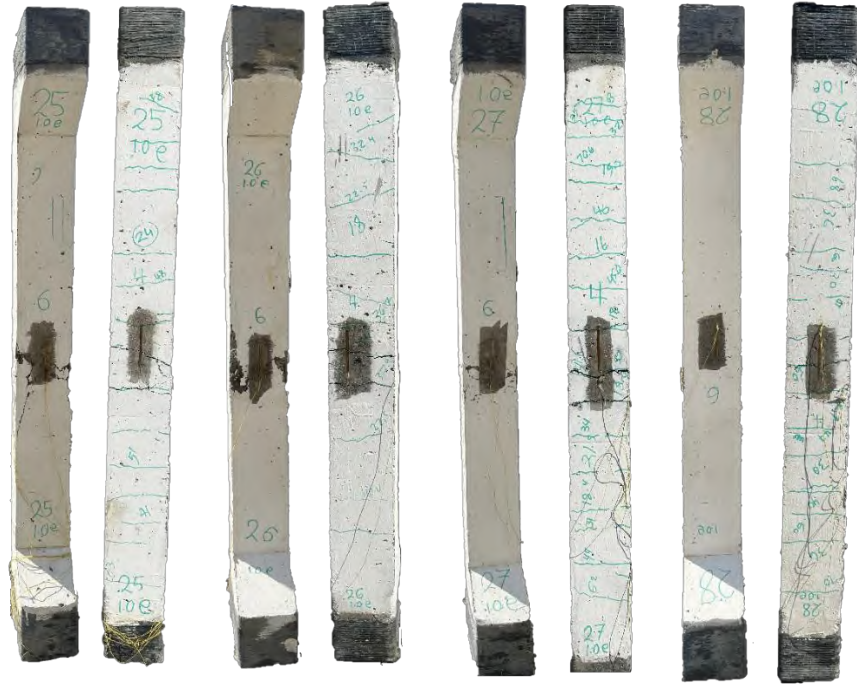
T-RA100Vf0E1.0 T-RA0Vf0E1.0 T-RA100Vf1E1.0 T-RA0Vf1E1.0 Figure 4.10: Failure mode of eccentrically loaded slender columns ( Kl/r = 26 , e/h = 1.0 )
