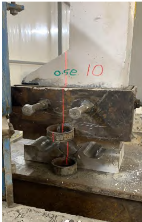
Figure 3.22: Pin support and laser used for alignment.
