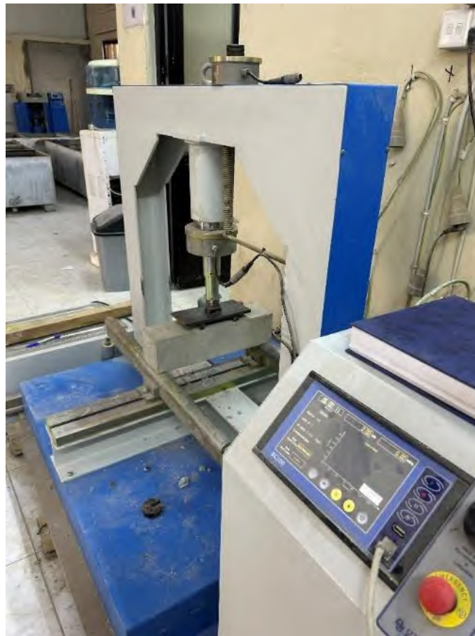
Figure 3.25: Hydraulic compression machine used for flexural strength of concrete.
