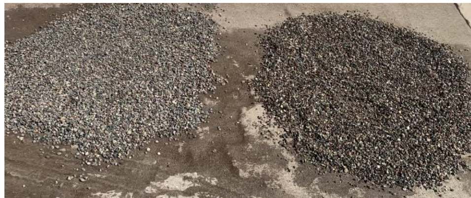
Figure 3.10: Coarse aggregate drying process: RA (left) and NA (right)
