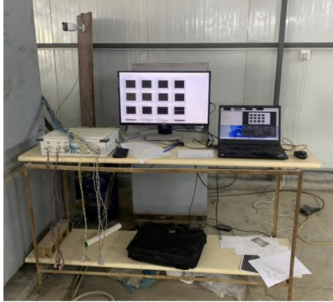
Figure 3.17: Equipment setup: computer, and data logger for sample testing
