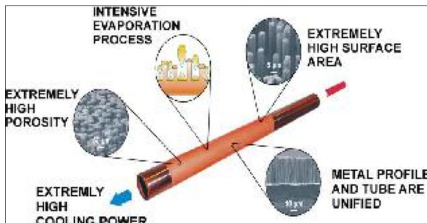
**Fig. 2.15** Microstructure whisker-attained copper tube (Schulz et al., 2005)
