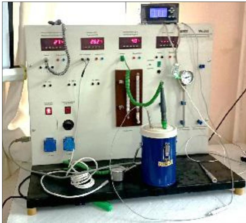
**Fig. A2.1** WL202 fundamentals of temperature measurement (GUNT)
