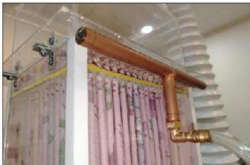
**Fig. 4.17** Dedicated water distribution system for proposed DPEC
