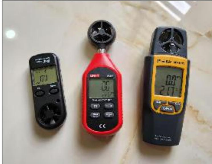
**Fig. A2.4** Employed anemometers for velocity measurement
