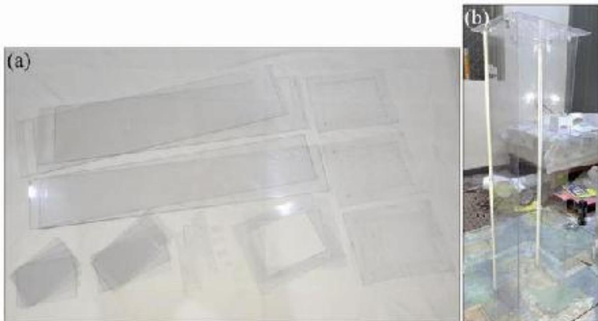
**Fig. 4.15** (a) Prepared acrylic sheets to compose the cooler's structure; (b) Cooler's structure reinforced with aluminum bars
