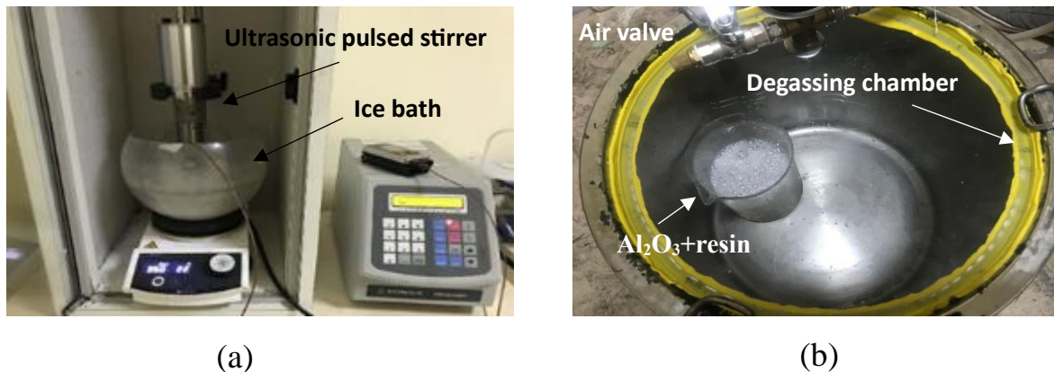
Figure (4.2) Aluminium Oxide Nanopowder ( \text{Al}_2\text{O}_3 ) and epoxy resin suspension mixing process, (a) UDMM, (b) Vacuum chamber degassing process
