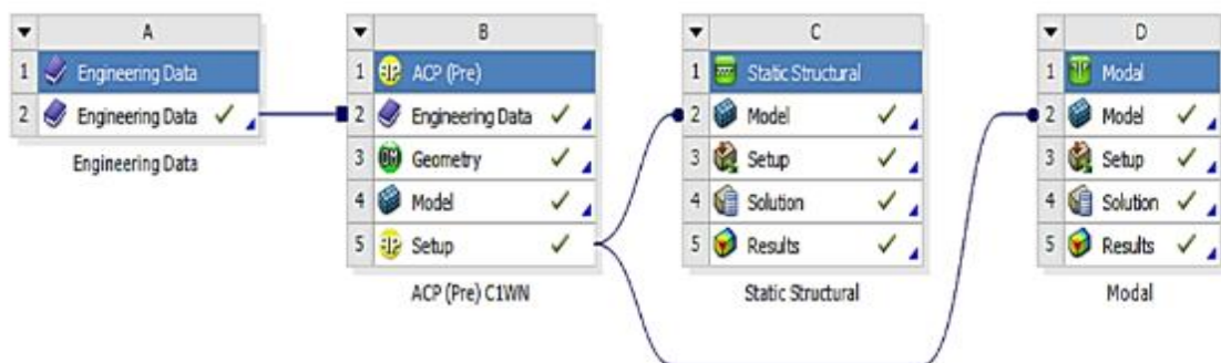
Figure (3.16) Steps of modeling orthotropic plate in ANSYS workbench to evaluate deflection and natural frequencies.
