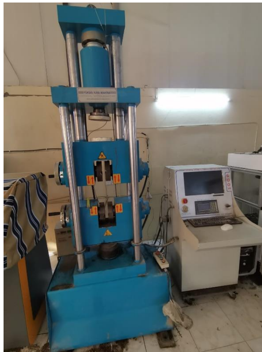
Fig. 3- 6 Hydraulic machine for tensile test
