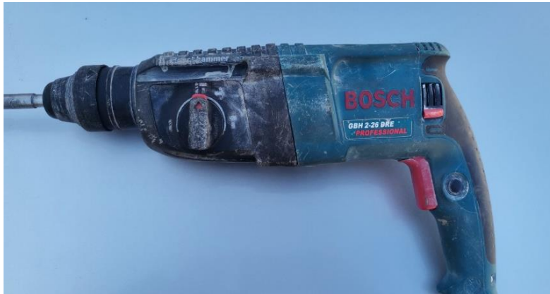
Fig. 3- 10 Rotating drill hammer drill
