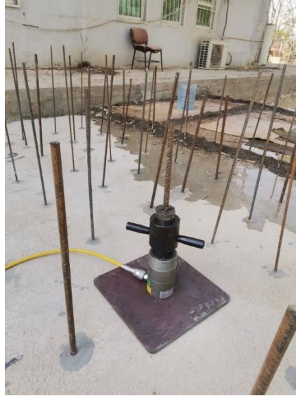
Fig. 3- 16 Pullout test configuration
