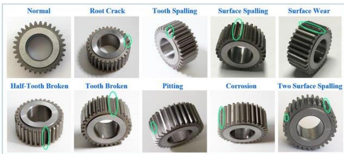
Figure 2.4: gear fault types(Jiao et al. , 2018).
