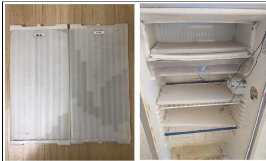
Figure 2.30. PCM configuration in the freezer and fridge cabinets (Karthikeyan et al., 2021).
