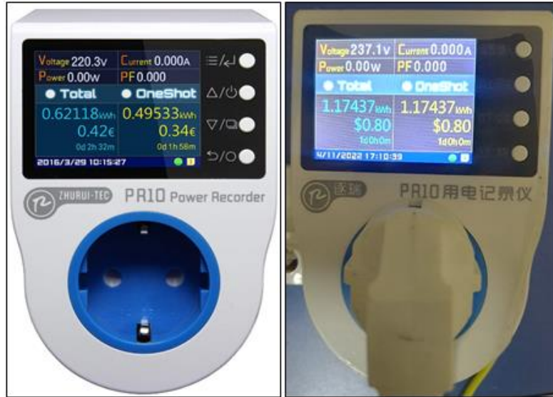
Figure 4.1. Zhurui power recorder (PR10) and its setup.
