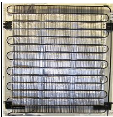
Figure 2.11. PCM configuration on the condenser by (Karthikeyan et al., 2021).
