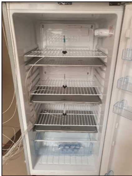
Figure 4.18. The position of aluminum PCM panels in the fridge cabinet.
