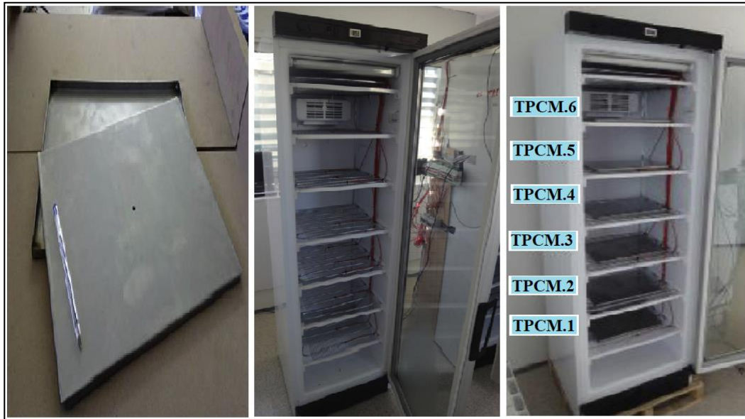
Figure 2.26. PCM encapsulation container and location by (Oró et al., 2012).
