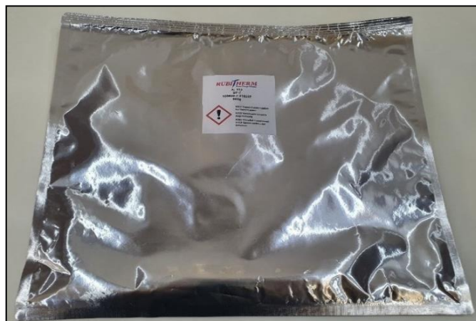
Figure 4.15. Rubitherm-manufactured aluminum pouches.
