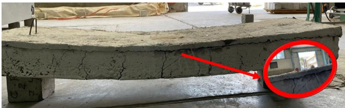
Figure 4.9: Delamination in a part width of S20 slab
