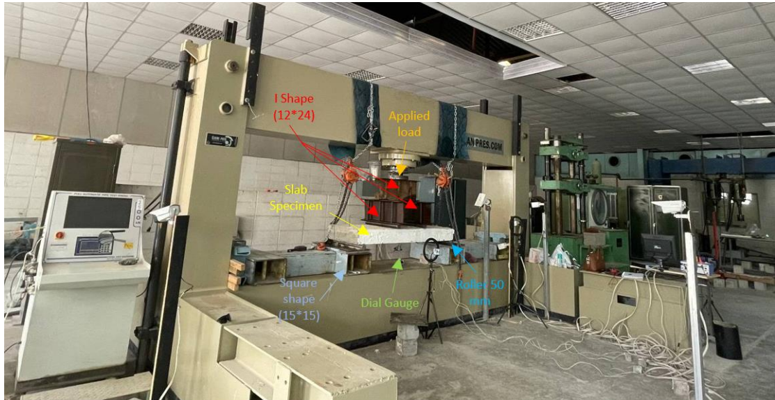
Figure 3.13: Details of the testing machine (Salahuddin university laboratory)
