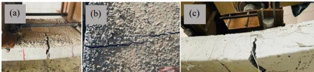
Figure 4.11: Failure mode of composite specimens: (a) Overlay f'_c 20MPa, (b) Overlay f'_c 80MPa and (c) Overlay f'_c 125MPa
