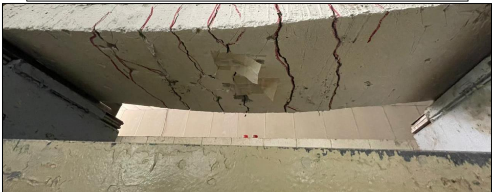
Figure 4.36: 3RA mold Crack pattern
