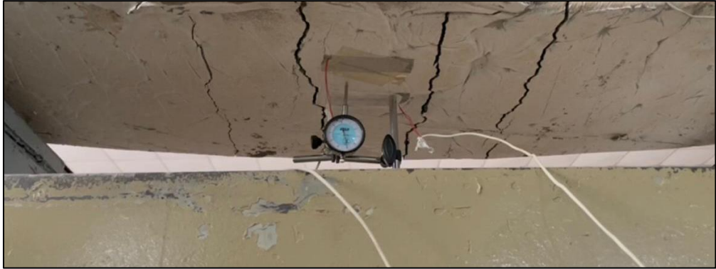
Figure 4.35: 2RA mold Crack pattern
